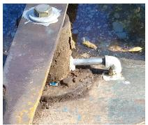
I had no trouble replacing the grease fitting extender using some black iron plumbing fittings and some JB Weld epoxy putty. But sharpening the blades was a bit more trouble.
