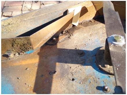
I noticed several bolts which stuck down into the clipping flow by about an inch. Silly. I cut them back with the mini grinder, flush with the nuts. You can see I swabbed up the spindle bolts and washers with anti-seize compound.
