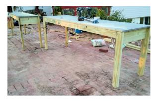
Importantly, both benches are 34" high, the same height as the top of my portable (thanks, Chris) table saw. This means that they can serve as material supports while feeding lumber or plywood through the saw. By coincidence they are also the same height as my extremely versatile
