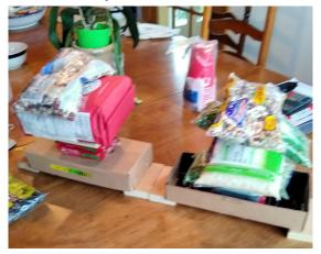
Watch the top edge of the girder in the bottom deck bridge for bulging indicating impending failure due to lateral buckling.
